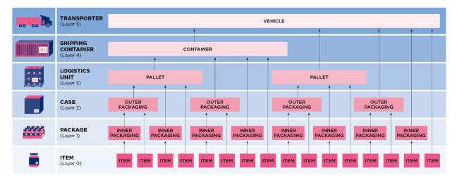
Figure 1: Typical Transport Hierarchy – example of cargo layers
